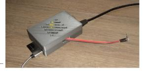
Simple MQTT temperature monitor
